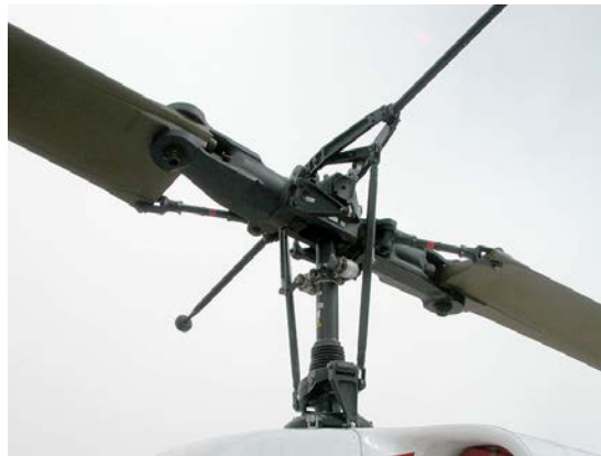
Figure 7: An example of a Semi-Rigid Rotor [5]
