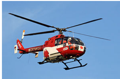
Figure 6: A MBB Bo 105 – an example of a rigid rotor helicopter [5]
