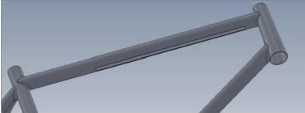
Figure 3 Close-up of top tube slit of aluminum frame
