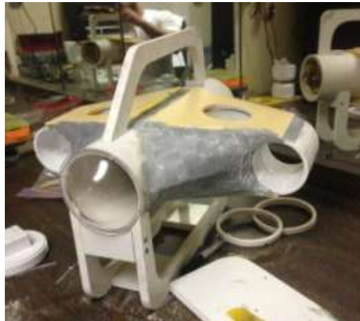
Figure 24. Cured Fiberglass and Polyester Resin
