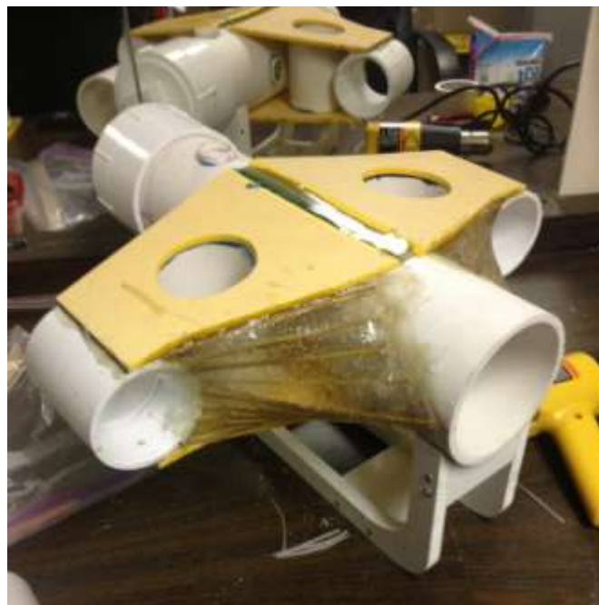
Figure 23. Application of Fiberglass and Polyester Resin
