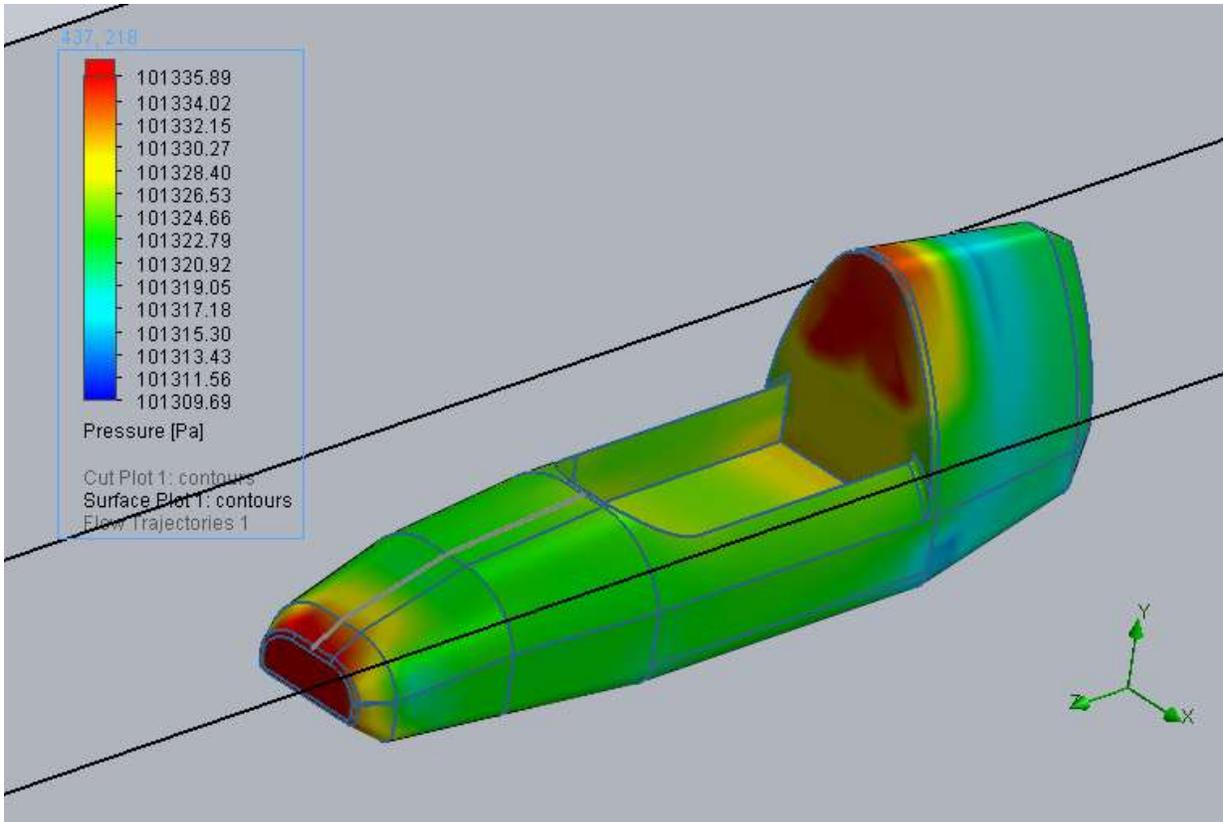
**Figure 11: Pressure distribution surface of the preliminary design concept alternative at 15 MPH (6.7056 M/S)**
