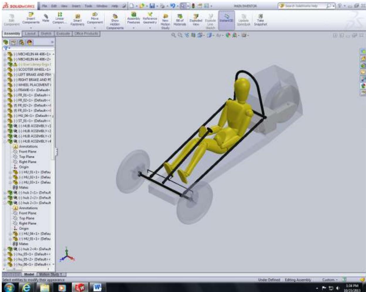
**Figure 9: Preliminary front end redesign components and driver cabin enlargement**
