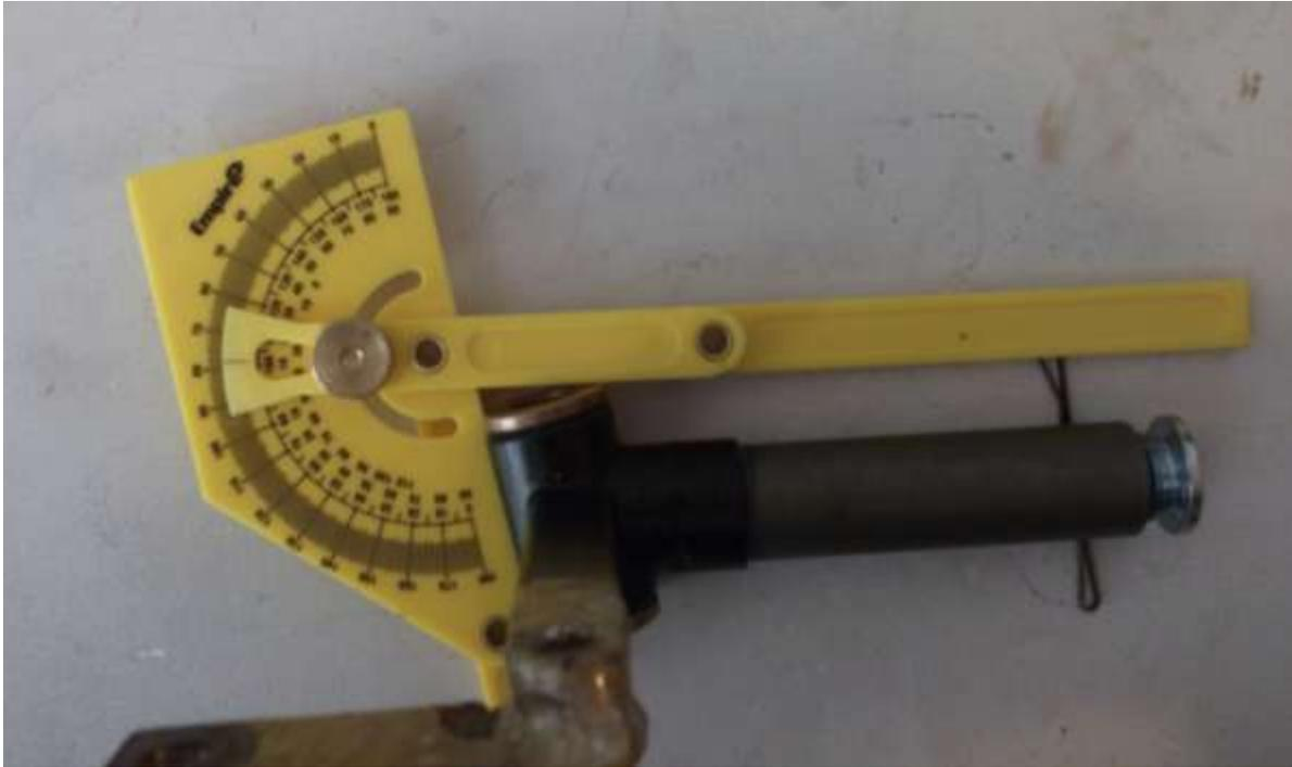
**Figure 5: The 12 degree offset hub that mounts the Michelin 44-406 20 inch tire and rim**
