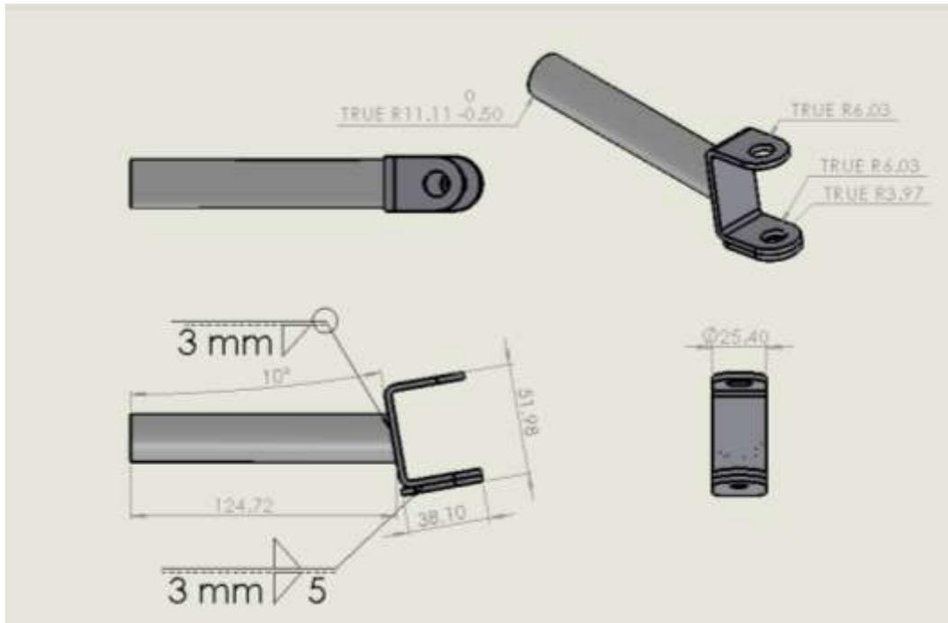
**Figure 7: The new 10 degree offset pivot that is currently being fabricated**
