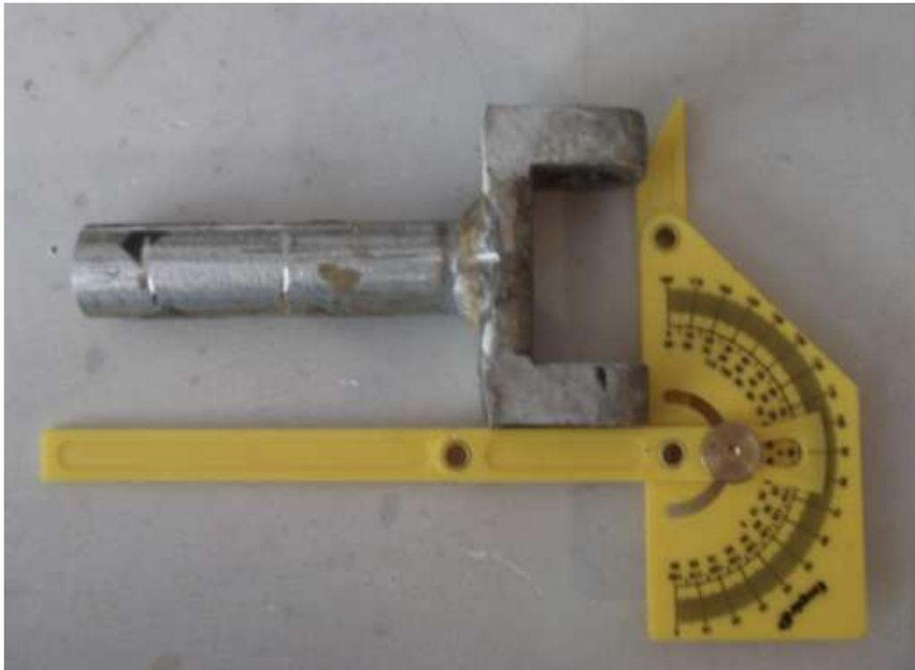
**Figure 6: The old 0 degree offset eco-marathon cart pivot that received the wheel hub**
