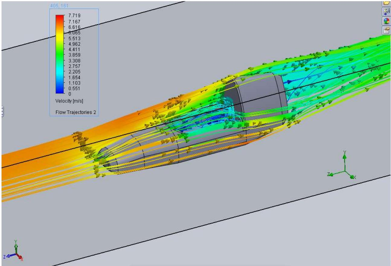
**Figure 12: Airflow across the preliminary design concept alternative at 15 MPH (6.7056 M/S)**
