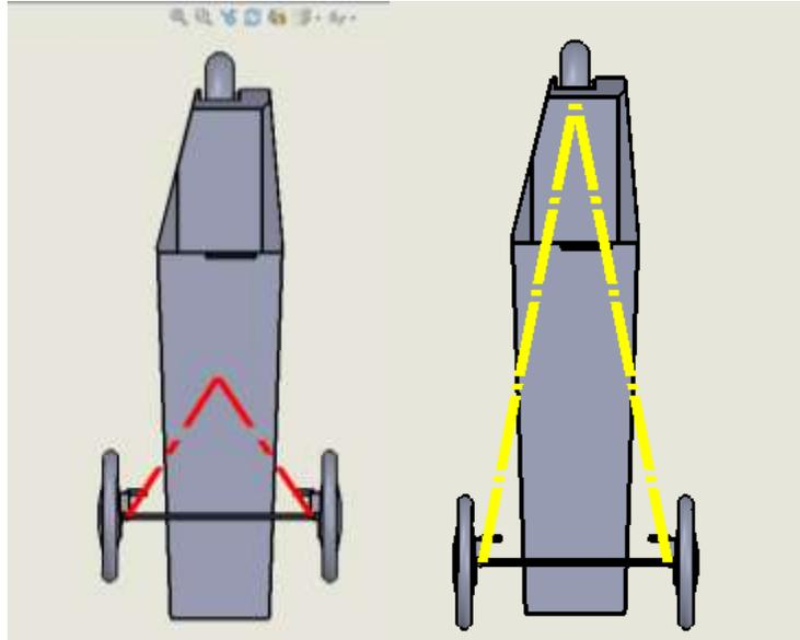
**Figure 4: Previous steering geometry (Left). Proposed Ackermann steering geometry design (Right)**
