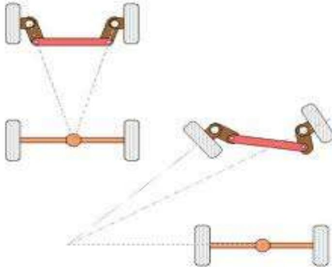
**Figure 3: Ackermann's geometry maintains turning radii with respect to the rear axle**
