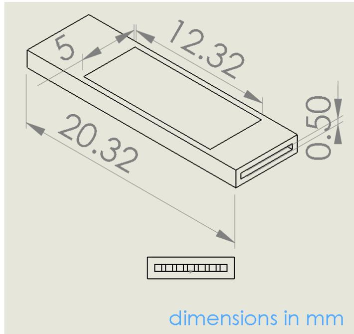
Figure 3 - Initial Design of Heat Exchanger
