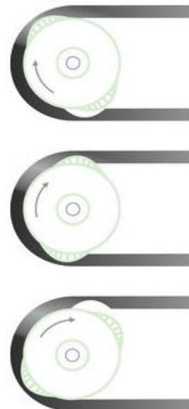
Figure 9: Peristaltic Pump Motion [06]
