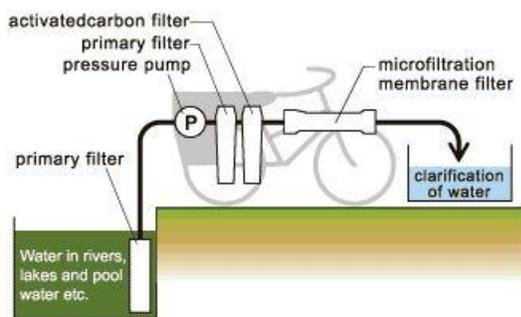
Figure 2: Schematic of Cycloclean [07]
