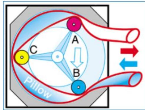
Figure 14: Peristaltic Pump Diagram [04]
