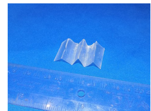
High surface area accordion type shape memory actuator
